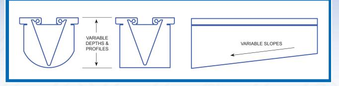
**MHD's** EPS foam former design flexibility allows the designer to select various system slopes, depths and section profiles to meet their specific requirements, site restrictions and hydraulics.
