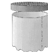
Standard grate only, used on smooth wall pipe.
