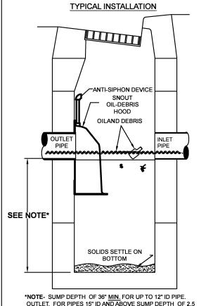
OUTLET. FOR PIPES 15" ID AND ABOVE SUMP DEPTH OF 2.5 TO 3 TIMES PIPE ID RECOMMENDED (E.G. 5' DEEP for 24" PIPE)
