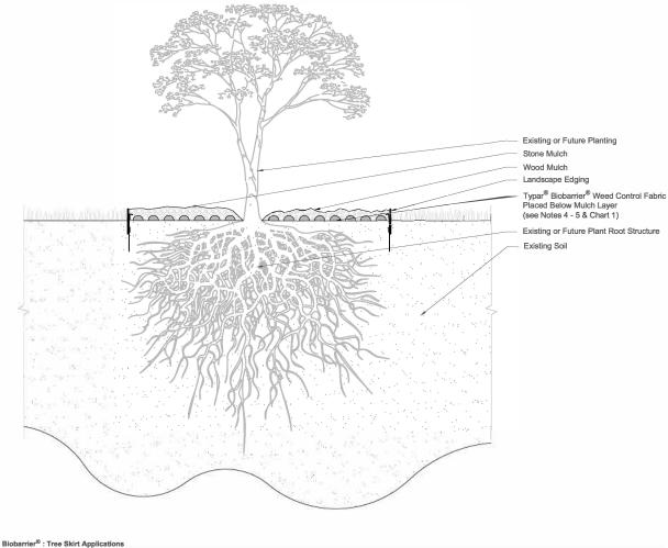
Chart 1 is a general guide only. Your specific applications may require slightly different sizes. As a general rule, the greater the fabric width, the greater the degree of protection against costly root damage. But, like any other root barrier the protection does not extend beyond the edge of the fabric. Soil's important to use adequate length and widthto assure proper protection.
