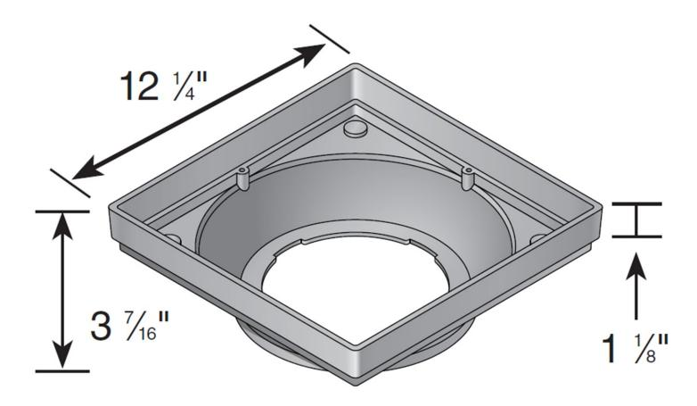
Part #: 1230 Material: (HIPS) High Impact Polystyrene Color: Black Fits: 3", 4", 6"or 8" sewer, drain and corrugated pipe, requires universal outlet #1243, #1245, #1266, and #1889. Use with 12" x 12" Grates Weight Per Each: 1.62 lbs. UV inhibitor
