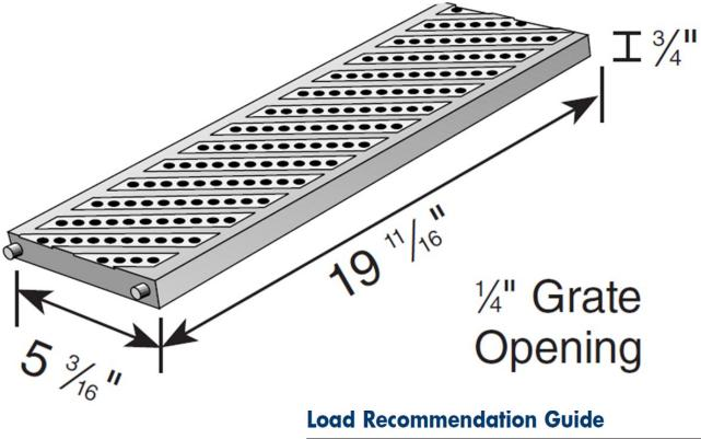
Part #: 826 Material: High Density Polyethylene Color: Light Gray Fits: 5" Pro Series Channel, Part# 820 ( takes 1 grate) and Part# 800 ( takes 2 grates) Grate Opening: 1/4" Open Surface Area: 4.86 Sq. Inch per Ft. Head Pressure / Flow Rate: <u>Head (inches) - Max Flow</u> 1" = 21.03 GPM 0.5" = 14.87 GPM Weight per each: 1.0 lbs. Screw: #829 Stainless Steel Screw, 4 per grate. UV Inhibitors
