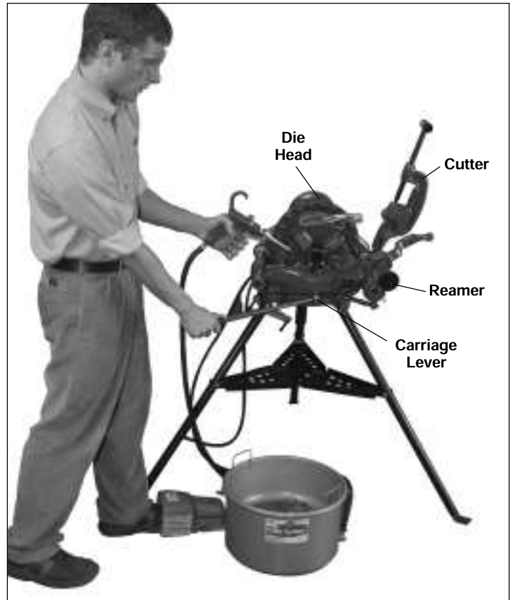
Figure 9 - Threading Pipe with R811 Die Head
