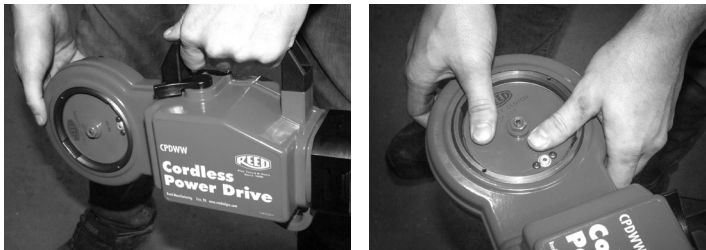
Note the orientation of the adapter to the CPDWW.
