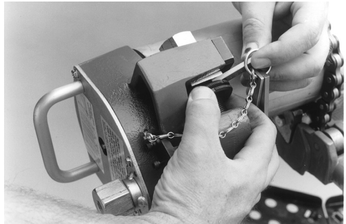
Fig. 3. Setting Gauge Depth
