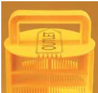
Figure 1: Arrow on top of filter unit must point in the direction of the outlet pipe. Top rim of filter will seat in hub of Tee.
