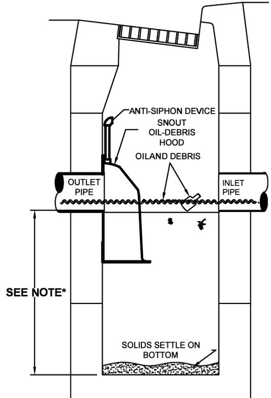
\*NOTE- SUMP DEPTH OF 36" MIN. FOR UP TO 12" ID PIPE. OUTLET. FOR PIPES 15" ID AND ABOVE SUMP DEPTH OF 2.5 TO 3 TIMES PIPE ID RECOMMENDED (E.G. 5' DEEP FOR 24" PIPE)
