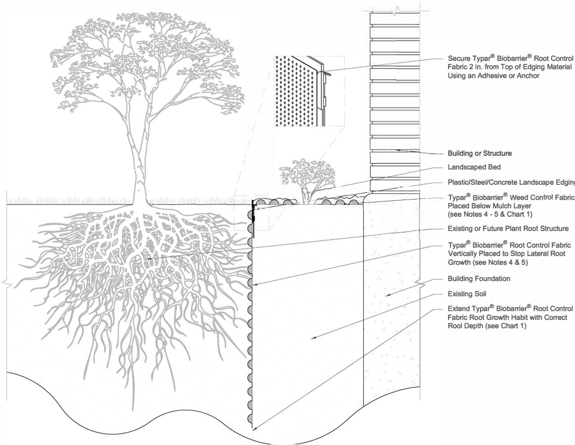
Secure Typar® Biobarrier® Root Control Fabric 2 in. from Top of Edging Material Using an Adhesive or Anchor
