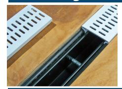
To stabilize a removable top deck drain, pin the base with 3/8" rebar (or like material) 3 to 4 foot on centers. Pinning the drain in this manner protects the drain from movement of concrete due to expansion and contraction.
