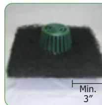
2. Verify size allows at least 3" of filter from outer edge of strainer.
