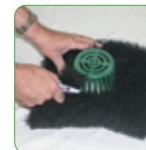
4. Slide Filter over strainer, net side down.
