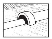
Test joint to engineer's specifications. Pressure test before backfilling or concealing. Bed and backfill properly.
