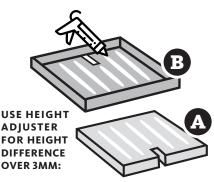
To calculate TOTAL adhesive to use with the Height Adjuster, remember there will be two lots of adhesive applied ie. adhesive is applied inside the Inlay Lid (B) AND the reverse side of the inlay material (A).
