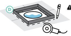
Ensure edge protector is centred over skimmer to mark cutting area. Allow for 1-2mm (1/16") clearance on all sides.
