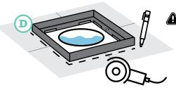
Ensure edge protector is centred over skimmer to mark cutting area. Allow for 1-2mm (1/16") clearance on all sides.
