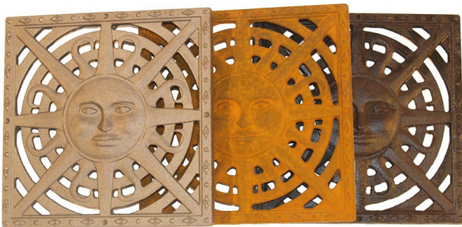
(Left) Raw cast iron grate; (Middle) Oxide layer (rust) forming after grate was sprayed with water; (Right) Rusty grate shown after application of Baked-On-Oil finish.
