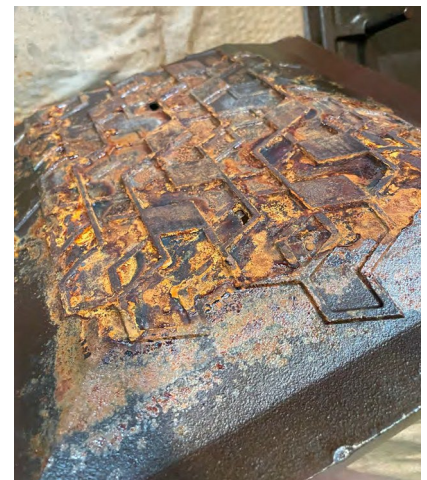
Baked grates stored outside in wet cardboard for a year.
