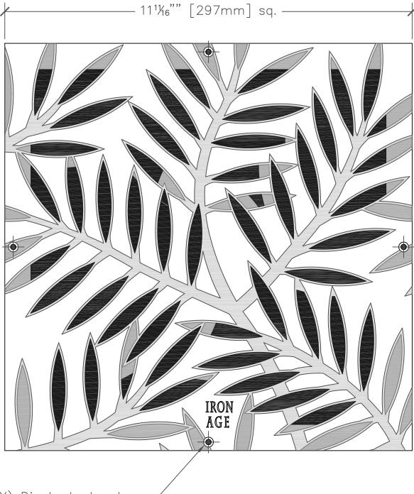
(4X) Divots to locate bolt-down holes as desired
