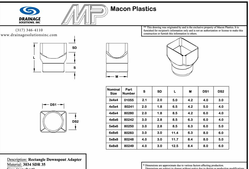
Dimensions are subject to change without notice due to design or production modifications. Unless otherwise specified, socket bottom to socket bottom dimensions are to be +/-1/2". Overall length dimensions are to be +/-1". All fitting angles are to be +/-1 degree. Outside dimensions are to be +/-1/4".
