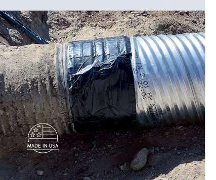
MarMac's CSP Coupler is a single unit, external sealing band which creates a flexible, strong, and permanent seal around the joints of corrugated steel pipe. The coupler is constructed of cross-laminated layers of rubberized mastic, integrated mechanical compression bands, an internal woven reinforcement, and butyl underlays.
