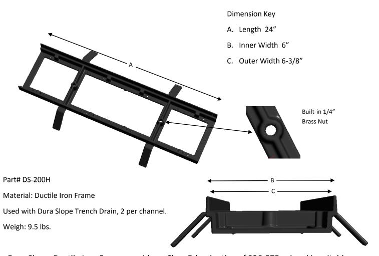
Dura Slope Ductile Iron Frame provides a Class D load rating of 326-575 psi and is suitable for heavy-duty hard tire equipment at speeds less than 20 mph. The DS-200 Ductile Iron Frame is recommended for use with pneumatic tire traffic such as fork lifts. The ductile iron frame can be used with the cast and ductile iron grates.
