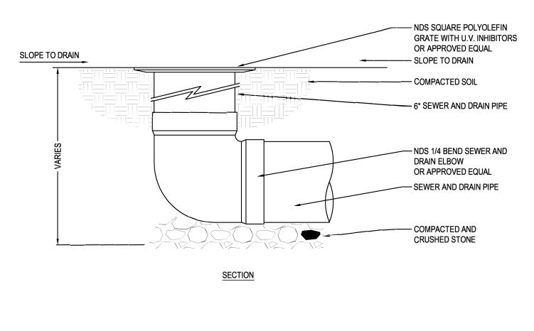
INSTALLATION TO BE COMPLETED IN ACCORDANCE WITH MANUFACTURER'S SPECIFICATIONS.
