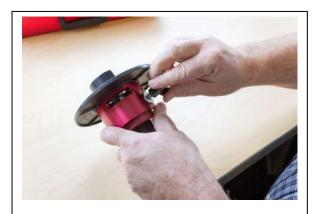
3. Replace washer. Insert adjustment knob and tighten completely.
