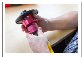
2. Slide adapter plate onto end of grinder and locate threaded hole/screw hole in the center of slot.
