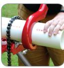
Protect plastic pipe with neoprene jaws or reverse for traditional steel jaws.
