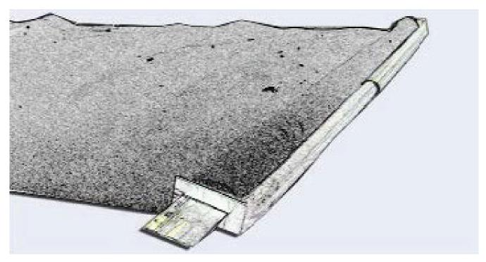
**Step 3:** Place flat ends of Straight Bar (A) through slots in ends of Locking Bar (B) and adjust to width of Dewatering Bag. Unit is now ready for use.
