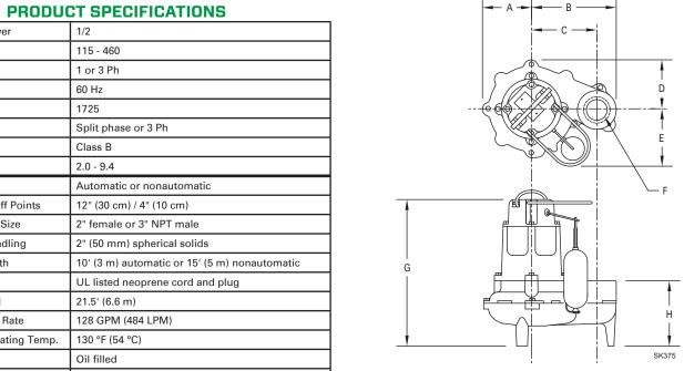
NOTE: The sizing of effluent systems normally requires variable level float(s) controls and properly sized basins to achieve required pumping cycles or dosing timers with nonautomatic pumps. See model comparison chart for specific details.
